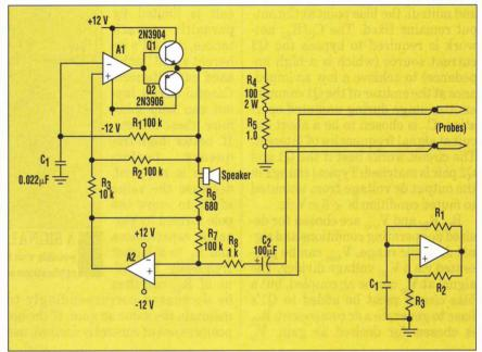
RESISTANCE BETWEEN BRIDGED TRACES can be translated into an audible tone with this circuit. The tone increases in pitch as the measured value approaches zero. The inset shows a classic op-amp multivibrator.
