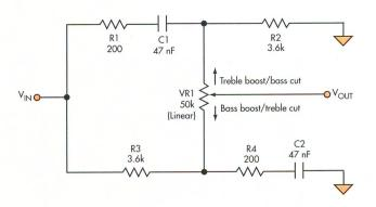
1. This simple circuit allows single-adjustment tone control for fine balance adjustment or applications where multiple controls are impractical.
