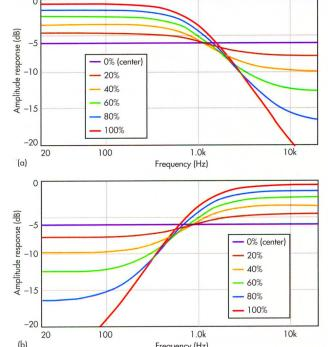
2. The tone-control circuit delivers good response characteristics in both the lower half (a) and upper half (b) of the control range.
